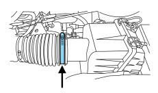
3. Remove the air cleaner assembly from the vehicle.
